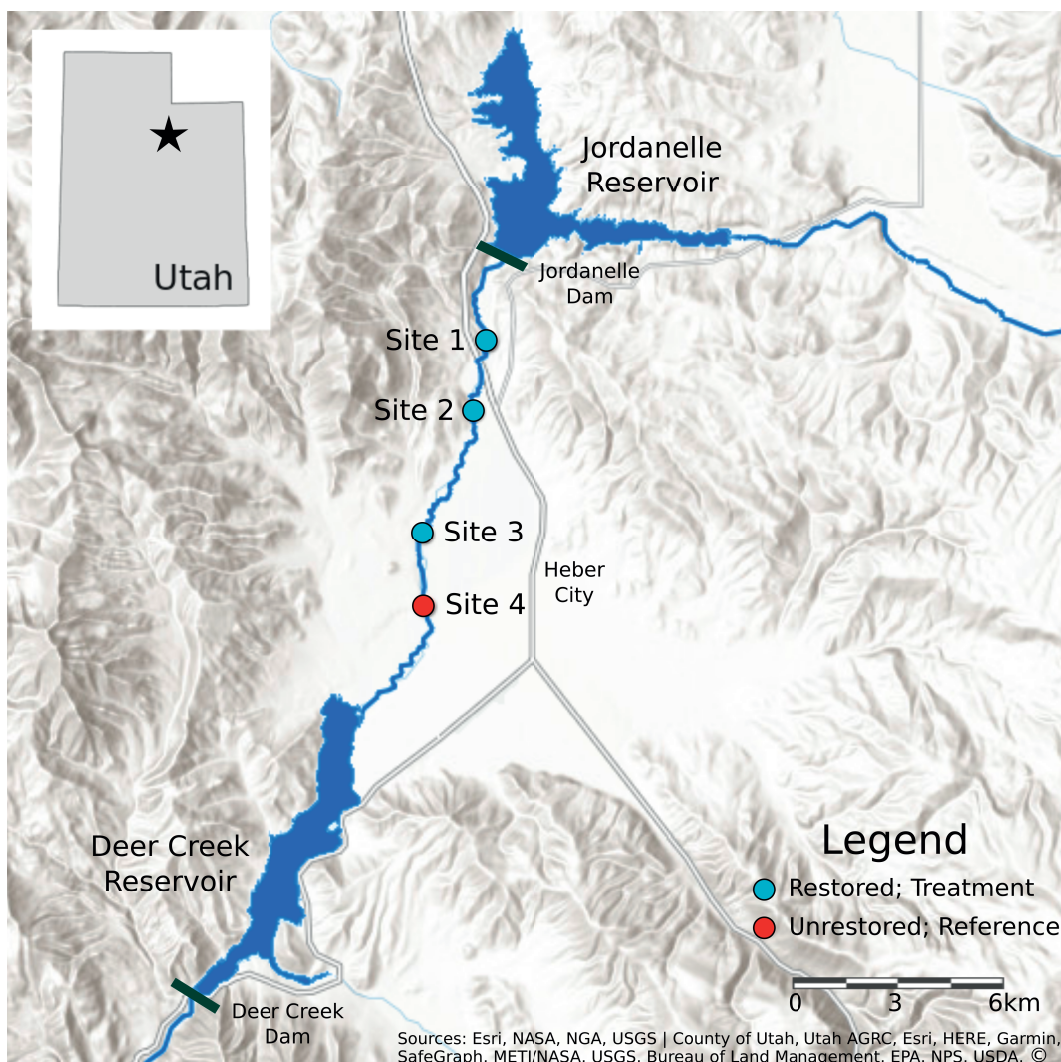
Fig. 1. The Provo River Restoration Project restored meanders and habitat heterogeneity to a 15 km stretch of the Middle Provo River, which had previously been channelized. Sites 1–3 (blue) lie within the restored segment and are referred to as treatment sites; site 4 (red) was never channelized or restored and is referred to as a reference site.
